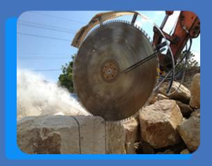
will cut to a depth that suits your needs. Each of our rock saws offers modern safety features including reversible blade spin, rapid automatic blade brakes and adjustable shields. The saws can be mounted on excavators from 1.7 tonnes up to 24 tonnes.
